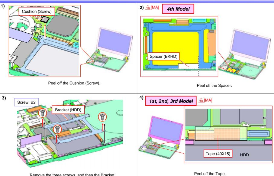
Remove the three screws, and then the Bracket.
