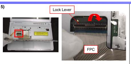
Release the lock, remove the FPC and remove the Keyboard. \* How to release the lock: Raise the lock lever toward the front.
