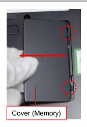
Hook a finger on the A portion, raise the Cover, and remove it in the direction of the arrow.
