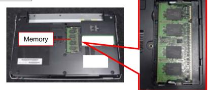
The Memory on side B of the Mother Board can be removed.
