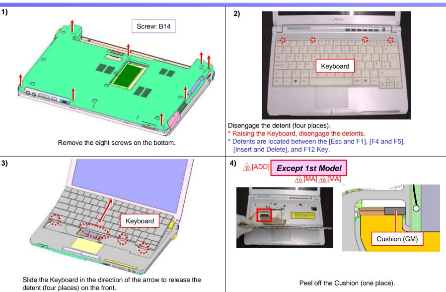
\* The FPC is connected on the backside of the Keyboard.
