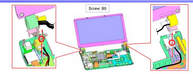
Remove the two screws, and then the LCD Section. \* Hold the LCD Section with your hand not to fall down. \* Release the coaxial cables from the main unit beforehand.
