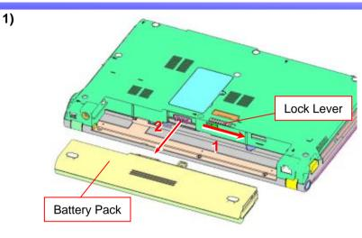
Slide the lock lever in the direction of the arrow 1, and remove the Battery Pack in the direction of the arrow 2.
