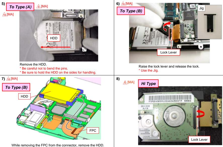
Raise the lock lever to release the lock. TX Series
